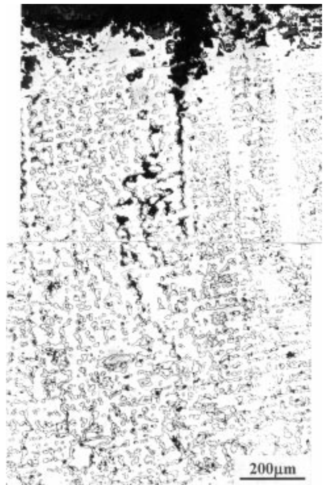
Fig. 4 Structure morphology on the cross section of the outer wall of the HP cracking tube
